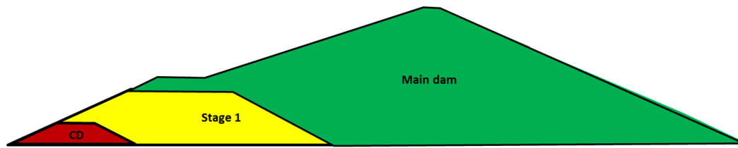
Figure 5: Dam Phasing used for Placement rate (2013, May)
