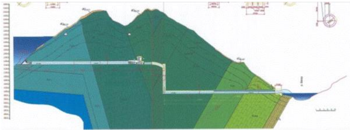
Figure 35 : 3rd operation spillway - longitudinal section
