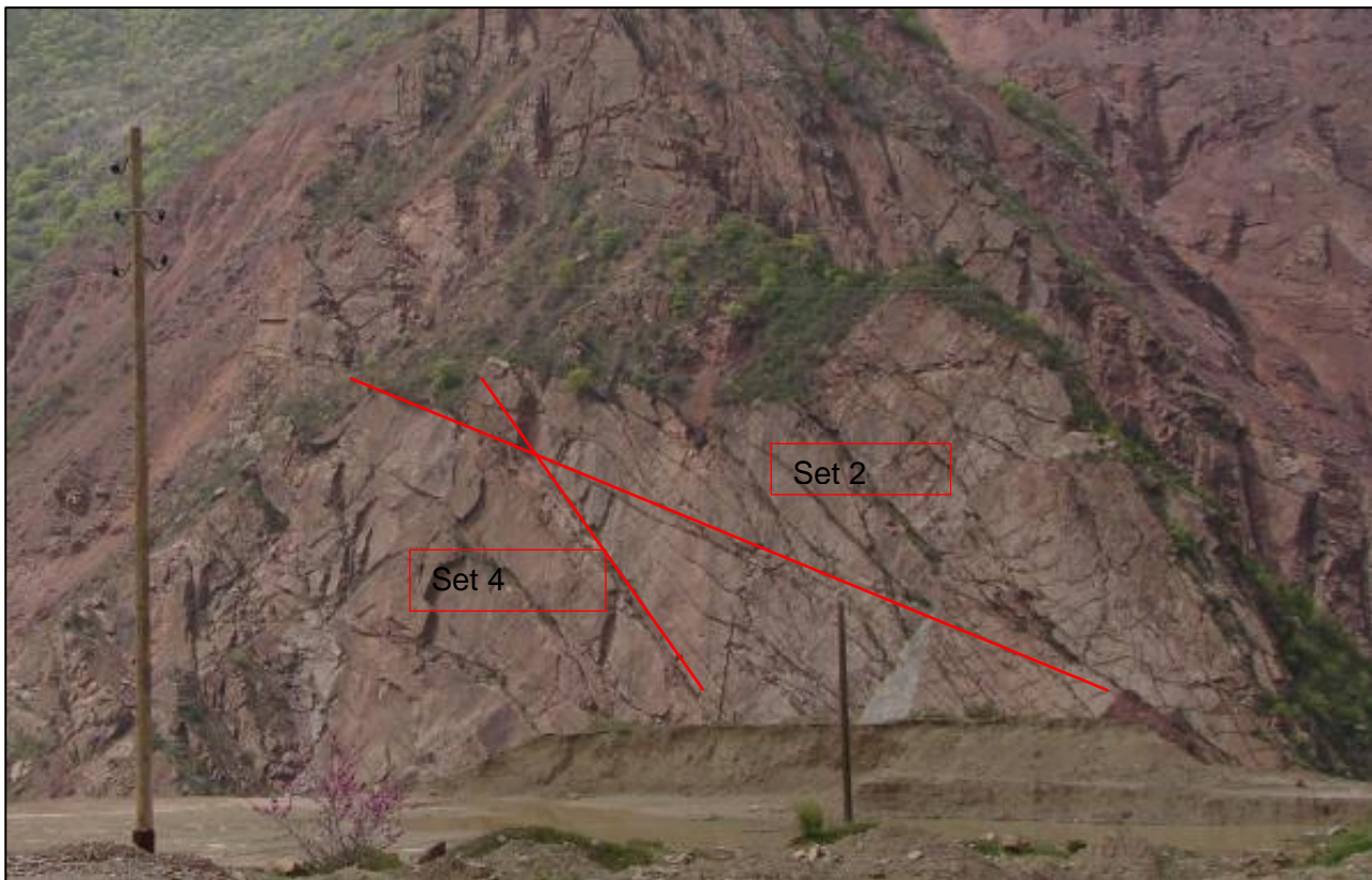
Figure 10.1: Photograph of the rock spur of downstream right bank, showing joint sets 2 and 4
