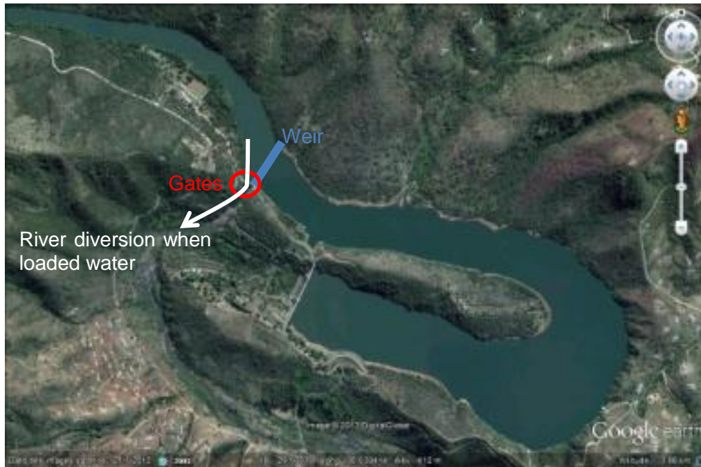
Figure 6.2 : Nadle dam (South Africa) - Reservoir by pass
