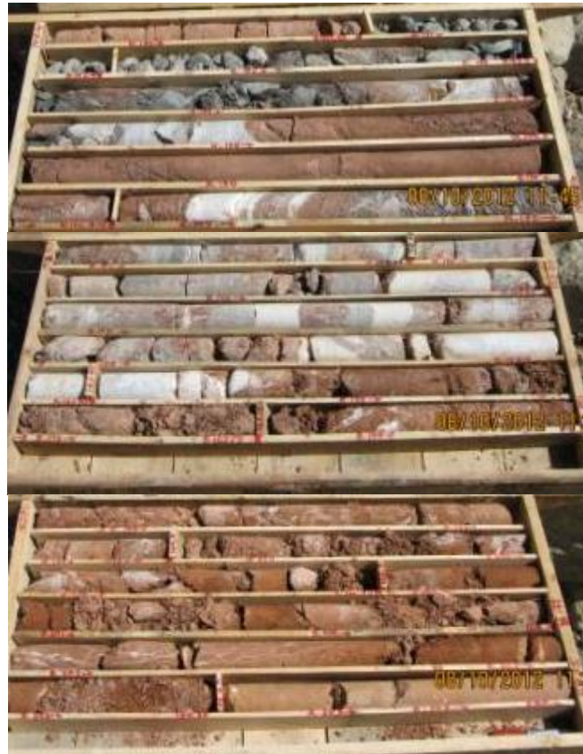
Illustration no. 18. Ionakhsh Fault zone in borehole WRB2
