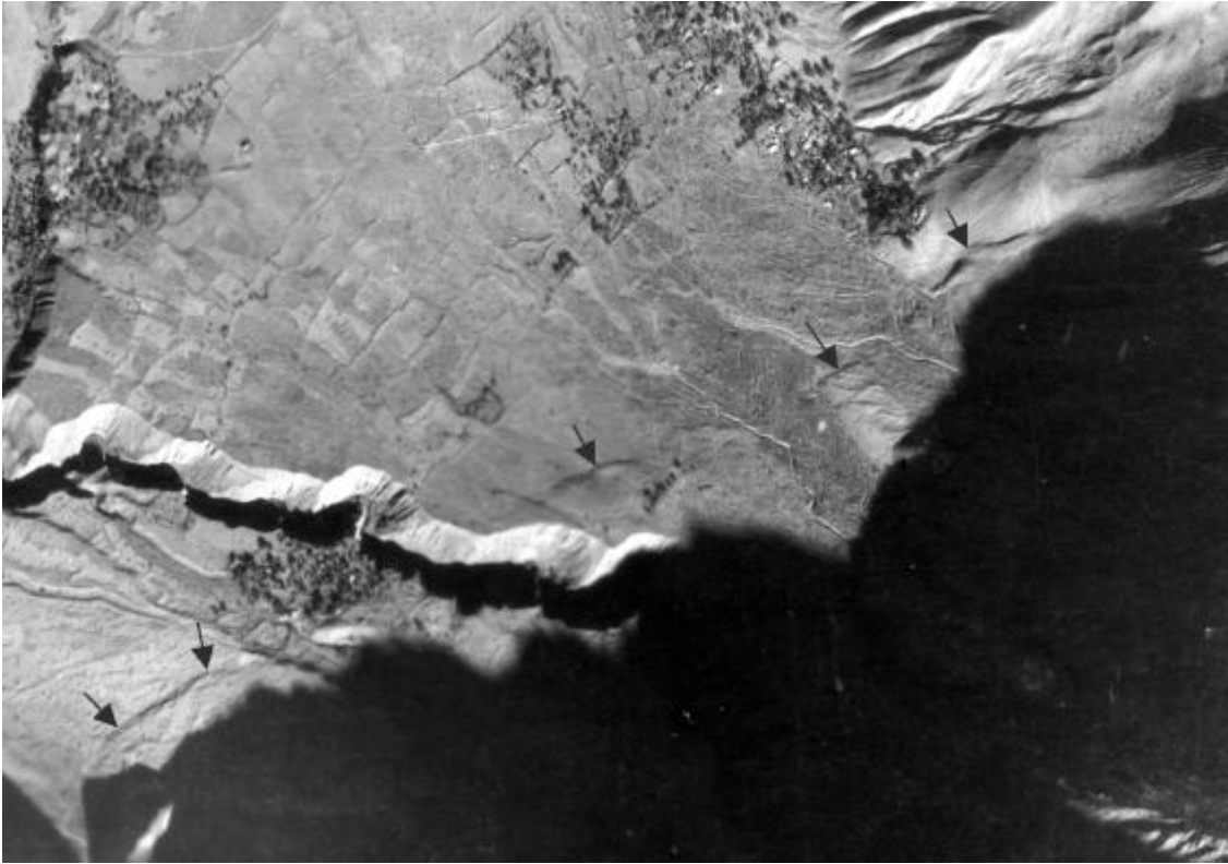
Illustration no. 46. Recent thrusts (arrows) near the foot of the Vakhsh Ridge in the area of Liabidar village.
