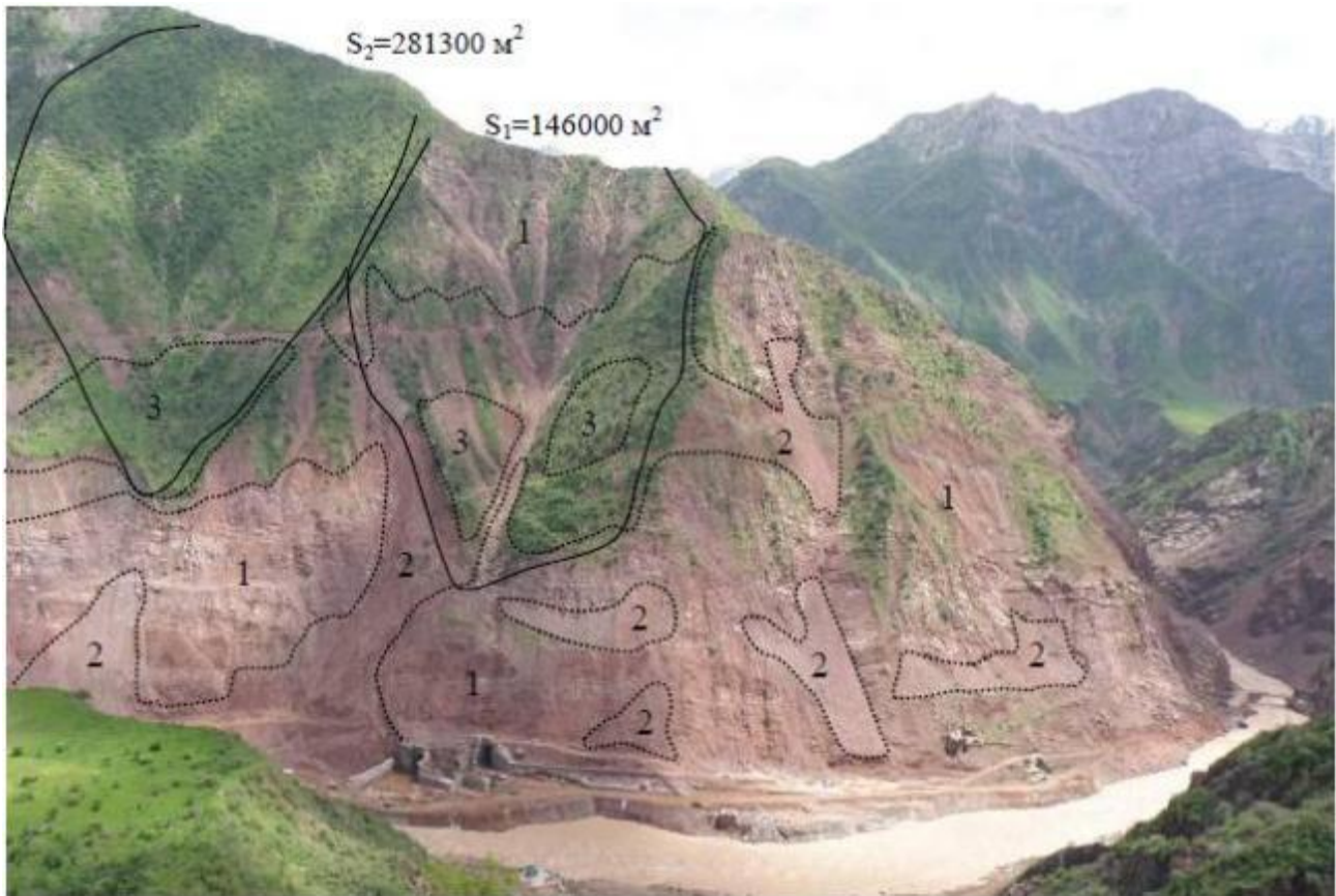
Illustration no. 30. Accumulation of thick slope deposits (3) in the upstream left bank.
