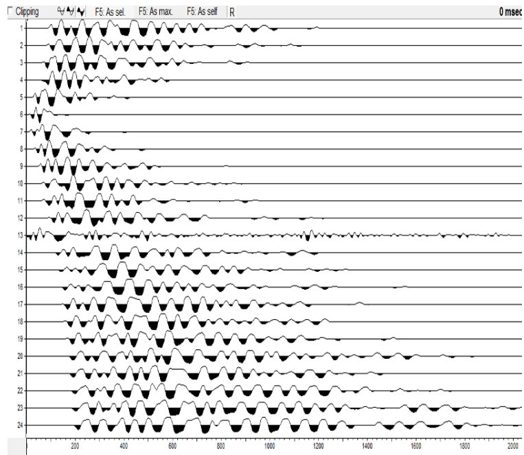
Fig. 25: Shot is located at 55 meters after the first geophone in the profile B of line 1
