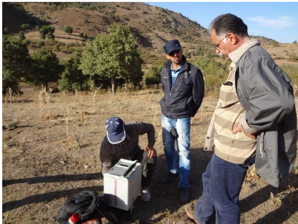
Fig. (6) : CG3 gravimeter used for data recording
