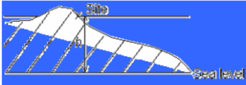
Fig. (5) : Schematic illustrate of free air correction effect
