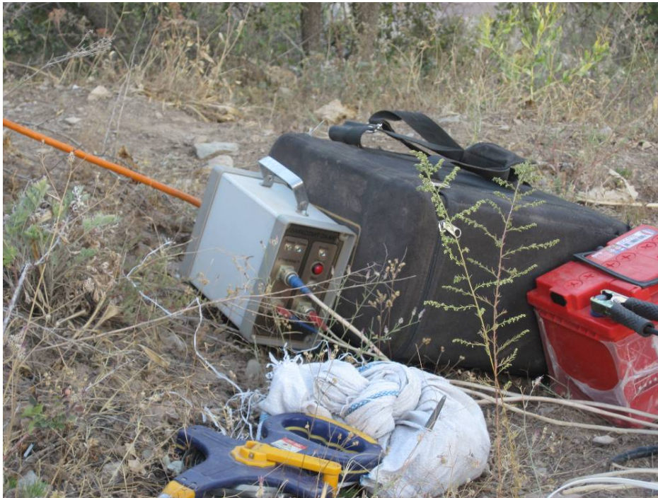
Photo 3: A view of the recording equipment used for refraction seismic surveys
