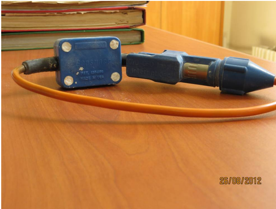
Photo 1: A sample of the geophones used for refraction seismic surveys at Rogun dam site
