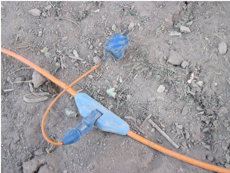
Photo 2: View of a geophone installed in the ground
