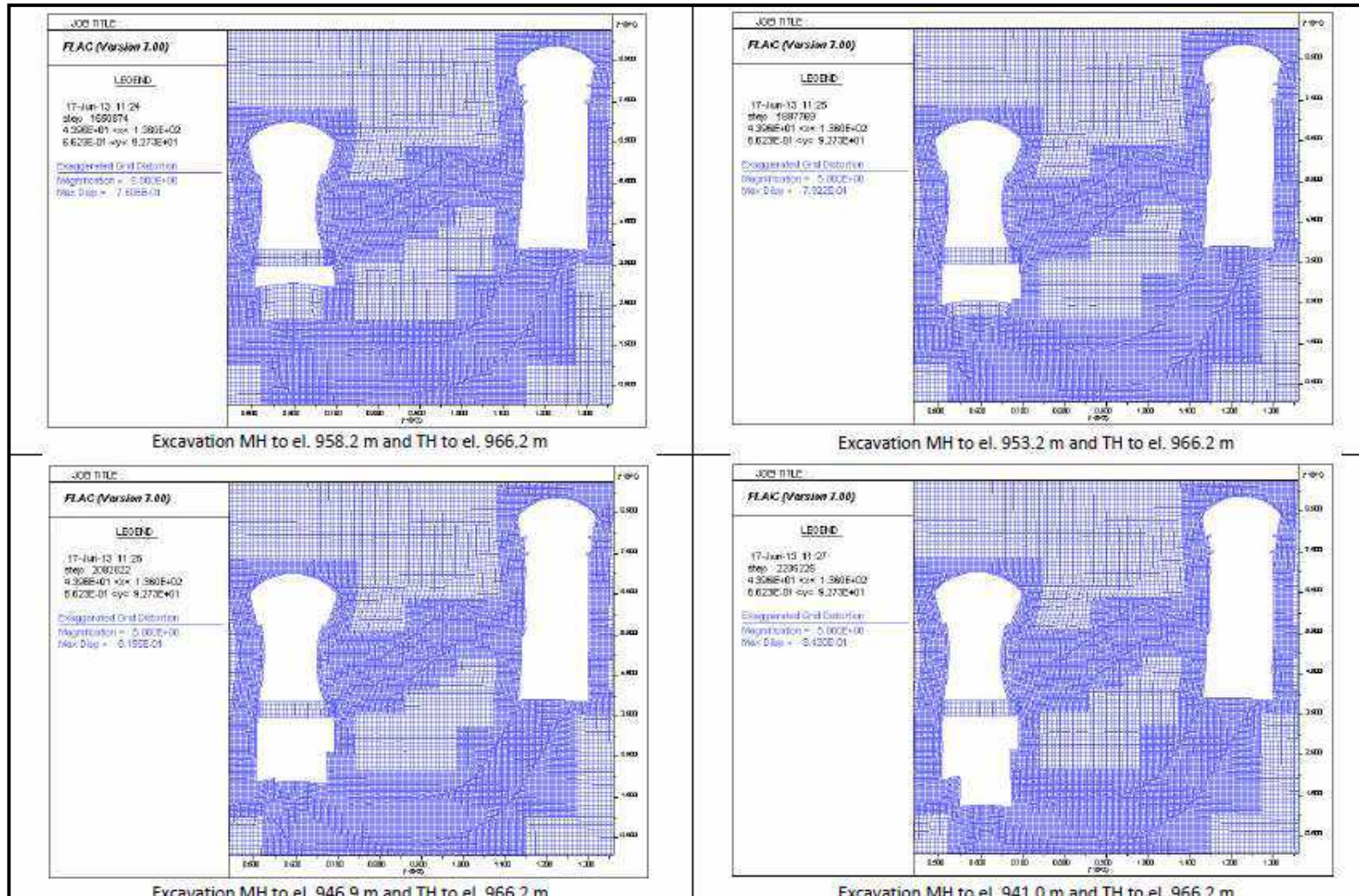
Figure 39: Illustration of deformed grid for excavation level in the MH cavern down to 941 m and in the TH cavern down to 966.2 m
